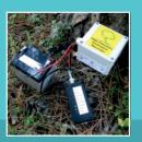
an instrument affixed to the root collar that measures the inclination of the trunk in two different directions. The instrument provides very accurate inclination data with sufficient frequency.
