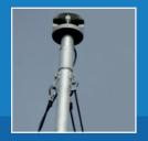
an instrument for measuring wind velocity at or near the tree to be evaluated. The closer to the better, but, depending on wind velocity DynaRoot may provide reliable data even with measurements taken several kilometres/miles away. The anemometer provides wind velocity data of sufficient frequency, Ideally the anemometer should be clear of buildings or other objects that may obstruct the wind, at a height of at least 10 m.
