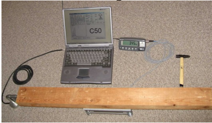
Fig. 4. The balance measures full timber load. Recommended setup for short (below 2m) lumber.
