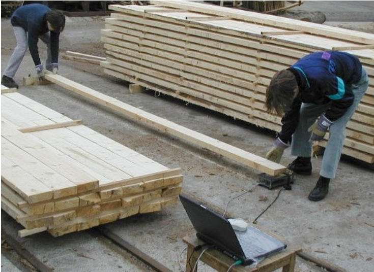
Grading soft wood lumber in a lumber yard.
