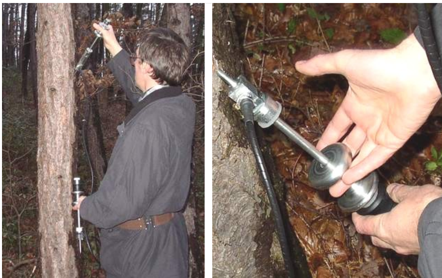
Figure 2. Driving the start (left) and stop (right) transducers into the tree using sliding hammer
