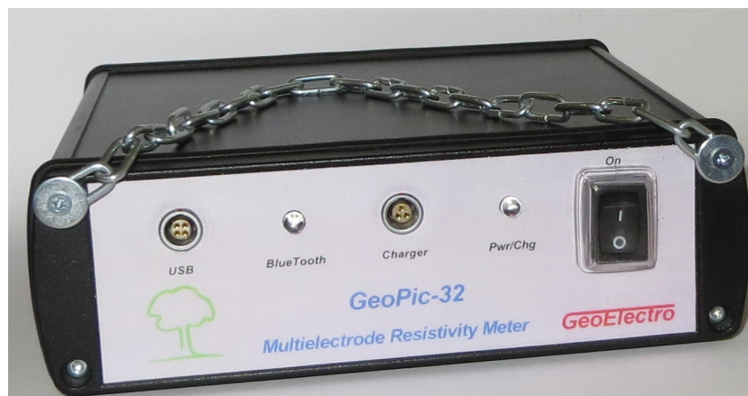
The front of the GeoPic-32 Multielectrode Resistivity Meter (without connection to the computer or charger)
