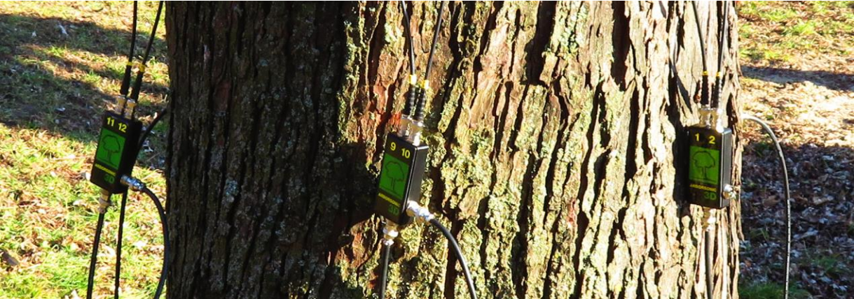
The Amplifier Box for sensors 9 and 10 was exchanged with the Amplifier Box for sensors 11 and 12. The tomogram has a hole and strange areas on the side.
