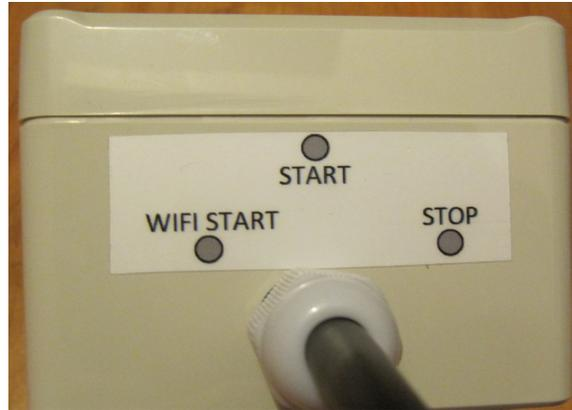
Figure 8: Touching the spots by the supplied magnet we can start and stop data collection or activate WiFi communication
