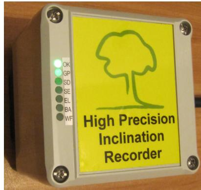
Figure 7: Inclinometer box with status LEDs
