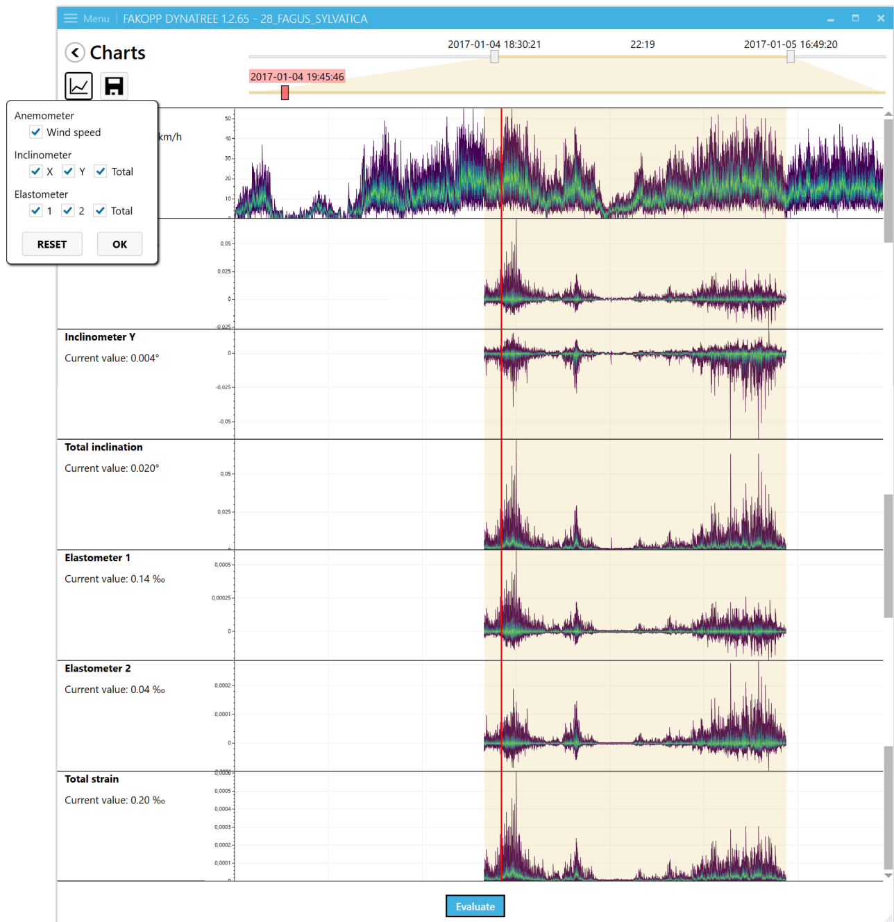
Figure 38: Wind speed, inclinometer and elastometer data can be turned on and off. As both inclination and elongation are measured on dual axes, the separated axes (like x or y directions) can also be presented. Total is for the whole inclination or elongation.
