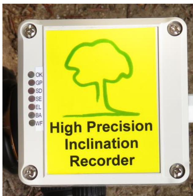
Figure 7: Indicator LEDs on the High Precision Inclination Recorder
