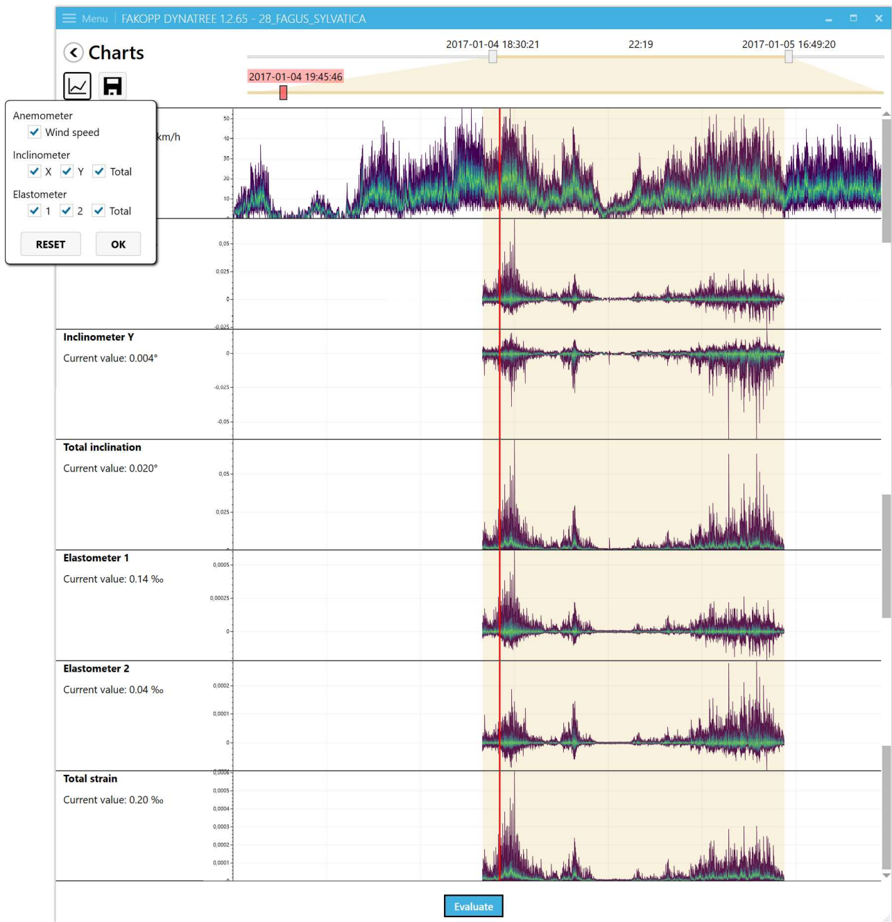
Figure 18 Wind speed, inclinometer and elastometer data can be turned on and off. As both inclination and elongation are measured on dual axes, the separated axes (like x or y directions) can also be presented. Total is for the whole inclination or elongation.
