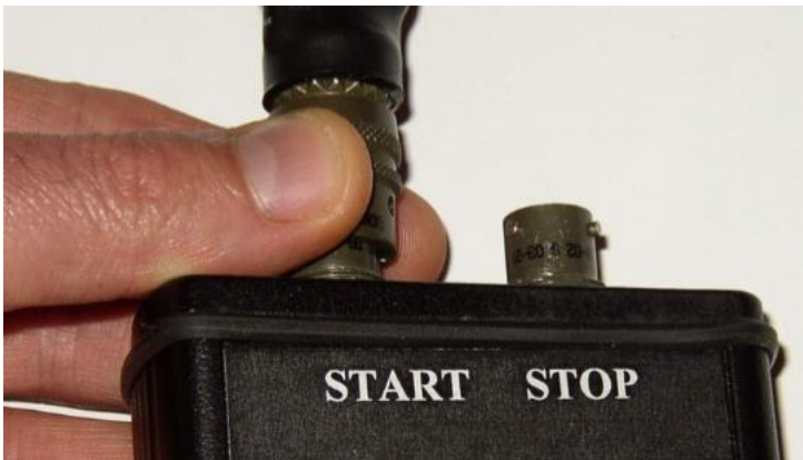
Figure 1. While connecting and disconnecting the transducers please touch the metal part only.
