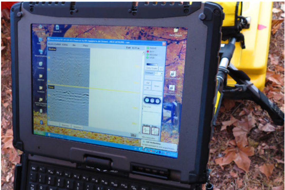
Figure 4.9. The screen of a GPR instrument. The measure itself does not require special skills – while interpreting the data usually requires both special software and experience. Source: own work
