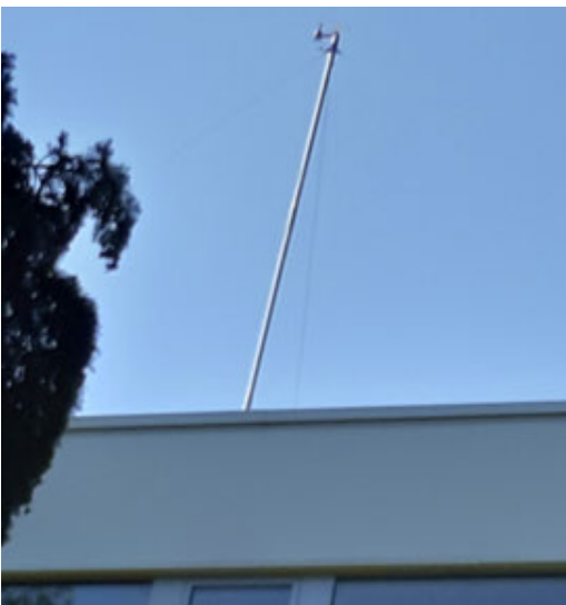
Figure 3.37. Anemometer permanently mounted on top of a building
