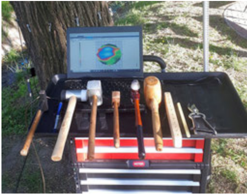
Figure 2.38. Tools used for sound generation
