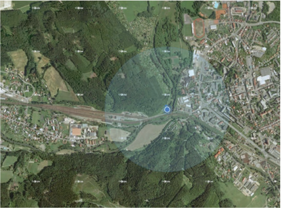
Figure 5.1. Area of error of a GNSS system shown on an aerial map
