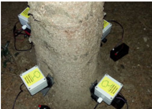
Figure 3.23. Using several inclinometers on the same tree
