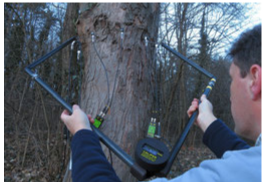
Figure 2.19. Using an electric caliper
