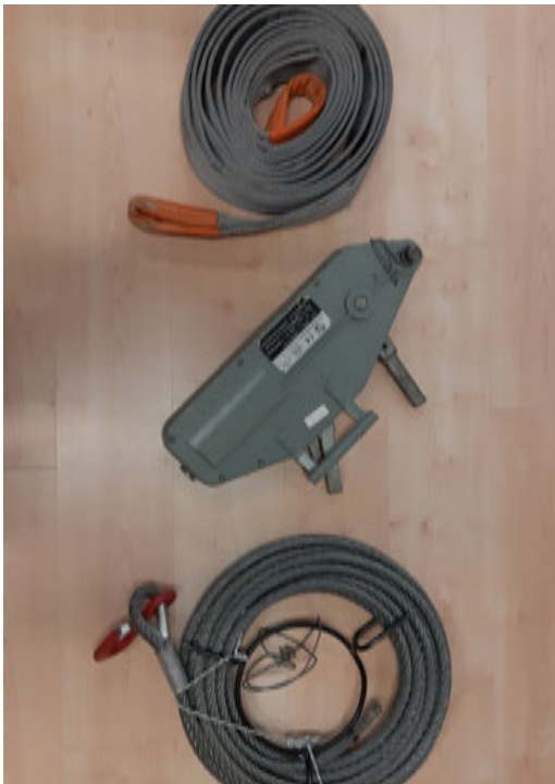
Figure 3.3. Cable, winch and strap used for creating lateral load on the tree
