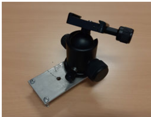
Figure 3.9. Mounting plate for inclinometer with biaxial levelling apparatus
