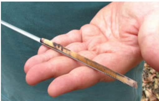
Figure 2.2. A (healthy) wooden sample in the groove, in the channel of the increment borer
