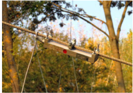
Figure 3.6. Cable-mounted calibrated load cell
