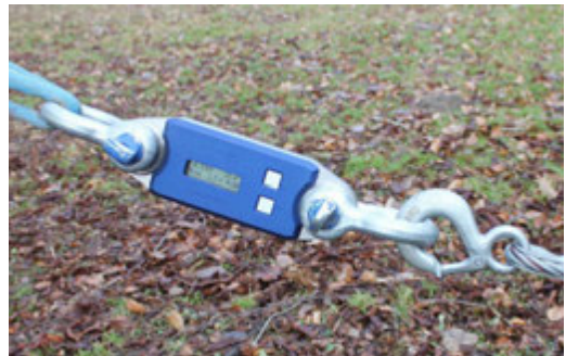
Figure 3.7. Load cell placed in-between the strap and the cable (courtesy of Argus Electronic GmbH)
