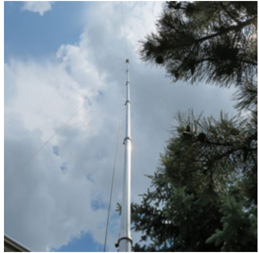
Figure 3.38. Anemometer mounted on mobile telescopic mast
