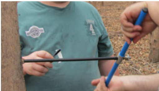
Figure 2.1. Sampling with increment borer
