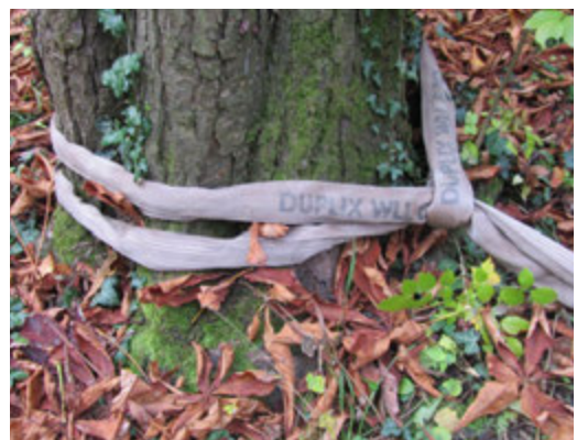
Figure 3.4. Using a strap to protect the tree
