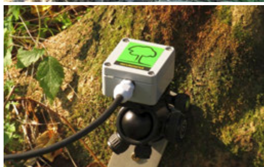
Figure 3.8. Inclinometers mounted on the root collar (courtesy of Argus Electronic GmbH and FAKOPP Ltd.)
