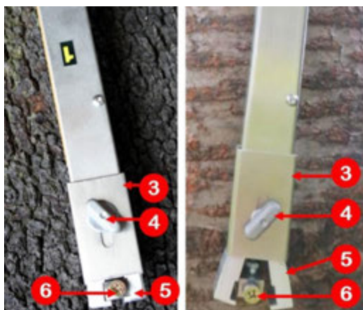
Figure 3.11. Extensometer in locked (left) and open (right) position. (1 – cable, 2 – casing, 3,4,5 – locking mechanism, 6 – moving core, courtesy of FAKOPP Ltd.)
