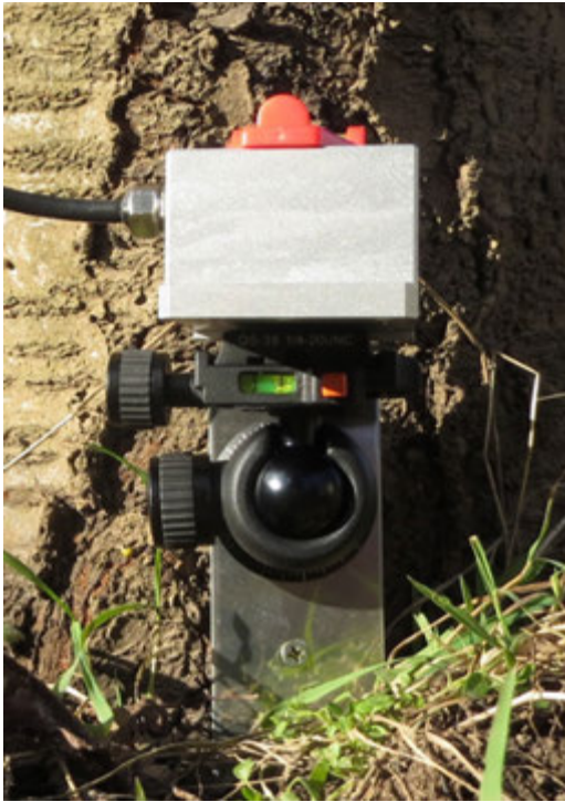
Figure 3.22. Mounting plate with built-in spirit level
