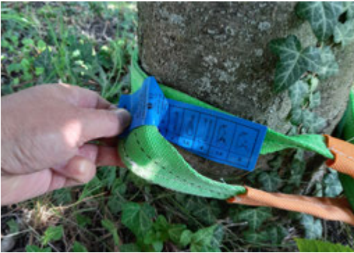
Figure 3.5. Checking the load rating on the protective strap
