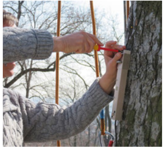
Figure 3.24. Mounting the extensometer on the side of the trunk, in the closed position
