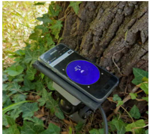
Figure 3.21. Levelling the inclinometer using a small spirit level (top) or a cell phone application (bottom)
